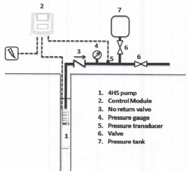
The control module receives the pressure signal from the pressure transducers and varies pump speed to maintain a constant set pressure regardless of water demand. In addition to the constant pressure control, CM can also the following control modes:
